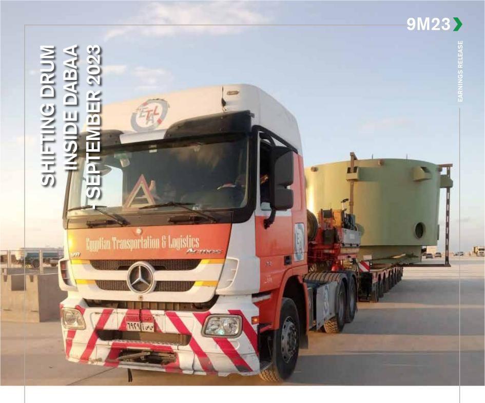
Shifting 1 Drum (7.10\*7.10\*4.15) inside Dabaa port using Superflex trailer.
